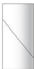
Type 4 Diagonal fracture with no cracking through ends; tap with hammer to distinguish from Type 1
